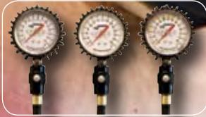
Liquid filled gauges have many advantages. But they can change readings by as much as 2-3 psi if the temperature changes . . .
