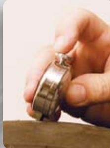
RECTANGULAR BASE straight edge keeps the durometer square with the tire for more accurate readings.
