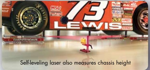
Self-leveling laser also measures chassis height
